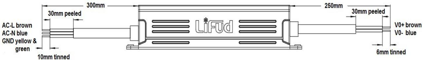
Cable specification: input 3\*17AWG/3\*1.04mm<sup>2</sup> (SJOW, H05RN-F) ØD8±1mm
